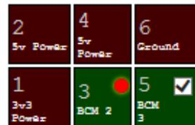
**GPIO.output** sends a value to an output pin
